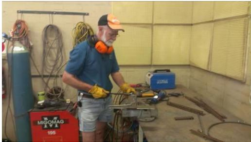
Then using a pram wheel as a jig to bend the rod into a circle to hold the water dish.
